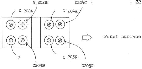
When this adjustment is made, a slight change takes place in input capacity. Accordingly, readjust the input capacity.
